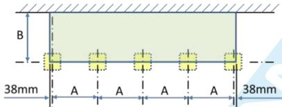
Rear Wall-plate face (fixed to adjacent wall/structure)
