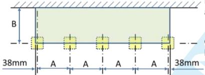
Rear Wall-plate face (fixed to adjacent wall/structure)
