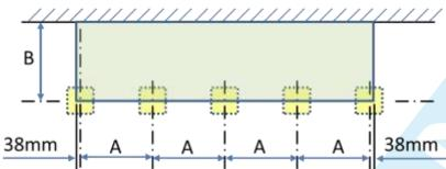
Rear Wall-plate face (fixed to adjacent wall/structure)
